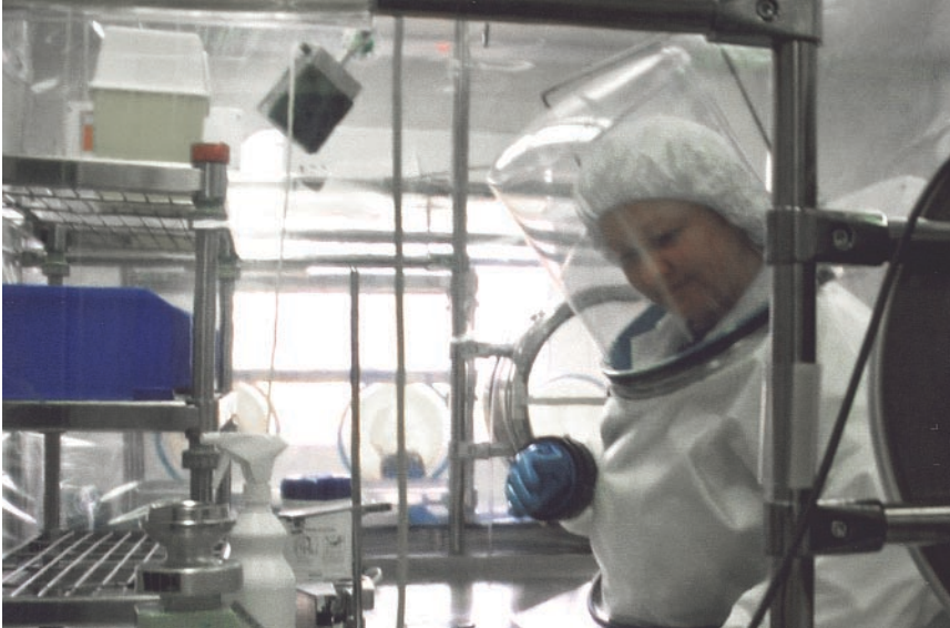
Technician encased in a half-suit isolator used to protect the small-batch test product.
