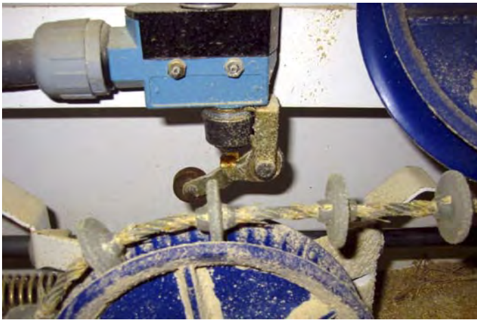
Photo #3 - Safety Switch (Roller Switch for Drive)
