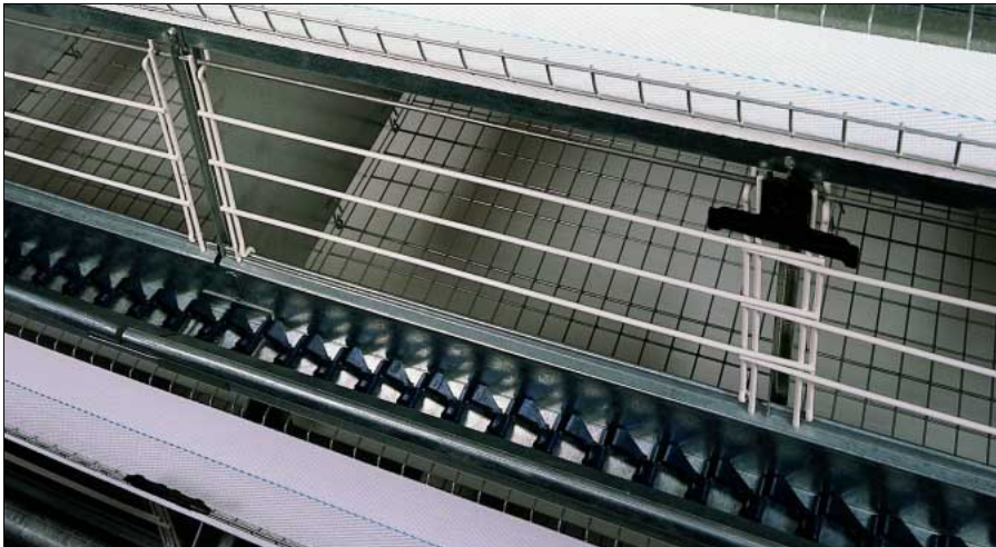
The CHAMPION feed chain distributes feed evenly, reliably and fast
