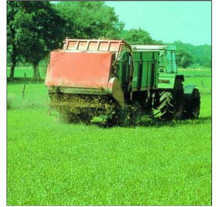
Dry manure is spread evenly using a plate-and-flicker distributor
