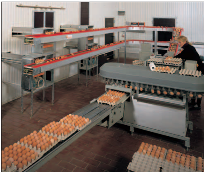
Eggs are transported to the farm packer via a curve conveyor
