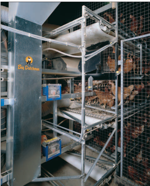
Manure belts collect the droppings
