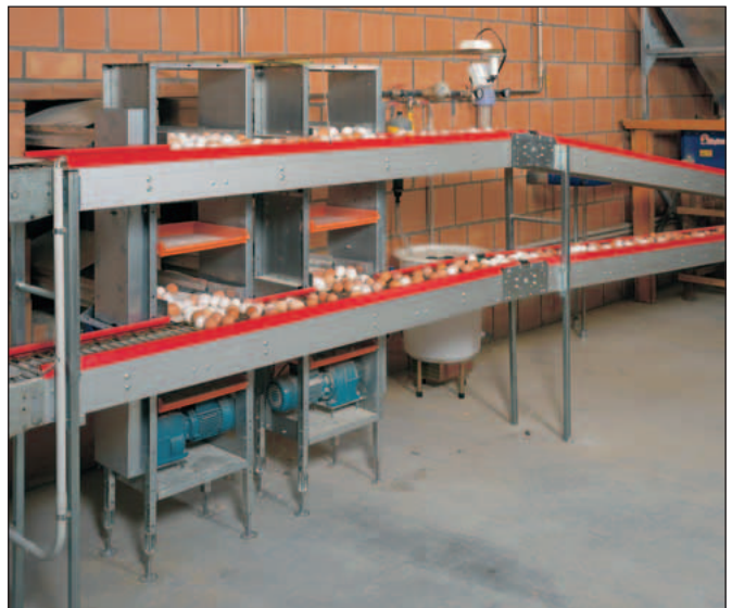
Egg transfer from the two-tiered Colony 2+ to a curve conveyor
