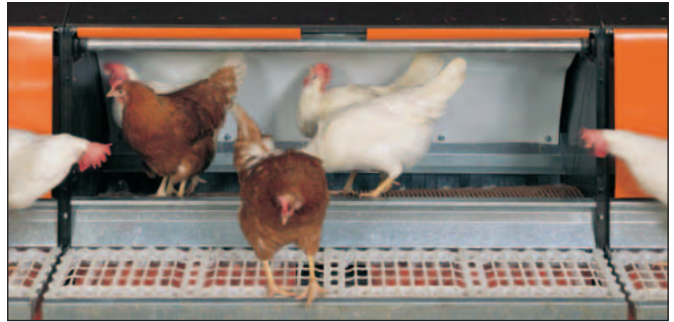
Colony 2+ – the group laying nest with patented tilting nest floor
