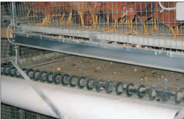
Manure belt underneath the supply area of NATURA-Floor
