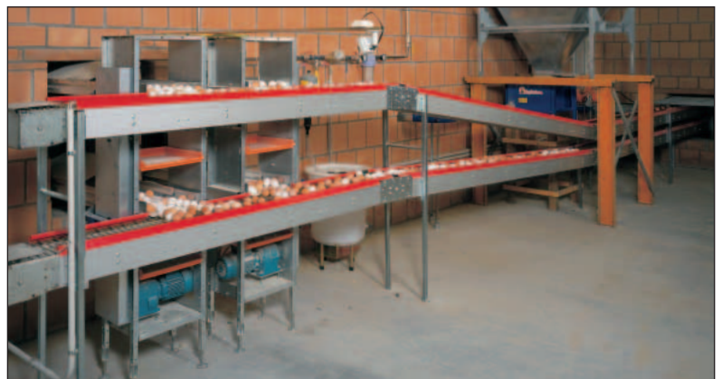
Transport of the eggs via a rod conveyor to the sorting machine
